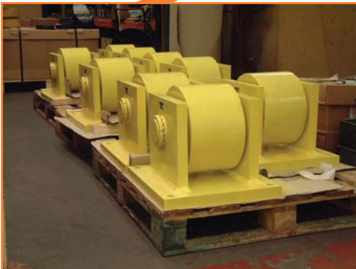
This ship mounted pipe laying turntable which is running on three rings of tapered tread steel wheels mounted in a fixed frame. The wheels and frame are finished in marine specification paint. Total weight when loaded is 600 tonnes with each wheel and bracket capable of carrying 50 tonnes.
